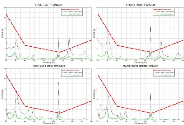
Figure 5: Hanging forces of the optimized model under engine load. The transmitted forces (black) compared to the design specifications (red) in the local Z-direction.
