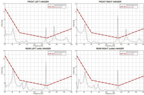
Figure 4: Hanging forces under engine load. The transmitted forces (black) compared to the design specifications (red) in the local Z-direction.
