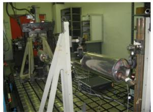
Figure 2: Exhaust system fixed on the test bench.
