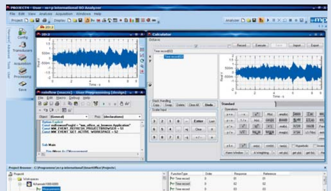
Advanced analysis of Coda data using m+p international's SO Analyzer
