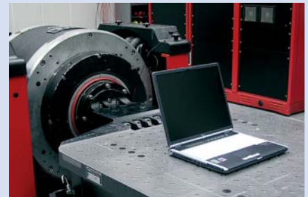
Vibration control at Fujitsu Siemens Computers, Augsburg/Germany
