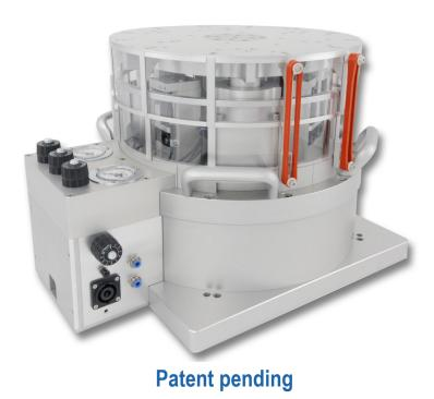
The **SE-13** Air Bearing shaker is an electrodynamic force generator specifically designed to be used for calibration and evaluation of accelerometers and other motion transducers in vertical direction. It provides excellent properties for low frequency excitation of such devices. The model consists of a large air bearing load mounting table that allows high payloads up to 50 kg (110 lb) e.g. for the calibration of geophones and heavy seismic sensors.
