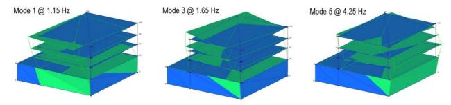
Figure 2. Mode Shapes of P block for OMA- Mode 1, Mode 3 & Mode 5
