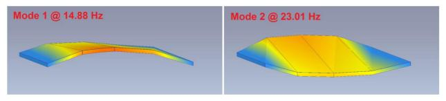
Figure 5. First two mode shapes of the foot bridge
