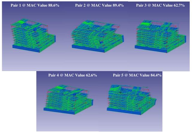
Figure 3. Comparison of FE mode shapes of updated model and OMA mode shapes of P Block
