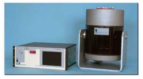
The LW-127-225 system is used when the test article size makes the ET-127 shaker the correct choice but test requirements do not demand the full rated shaker performance available from the LW-127-500 system.
