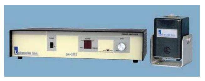
Specify the LW132-203.151-4.5 system when a light weight, portable system with maximum high frequency is desired for the general purpose testing and calibration of small components. This system is popular because of its low mass armature, high frequency capability, enhanced random vibration performance, and it is one of the smallest shakers available capable of DC (linear actuator) operation.
