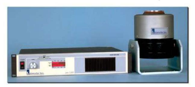
The LW139.138-40 system is an excellent choice for modal testing due to the small shaker size, large displacement and absence of cooling hoses. Due to its compact size, this system is highly portable. The power amplifier has the option of being operated in the current source mode to facilitate modal testing. The large armature table facilitates general vibration testing of components and subassemblies with the amplifier in voltage source mode..
