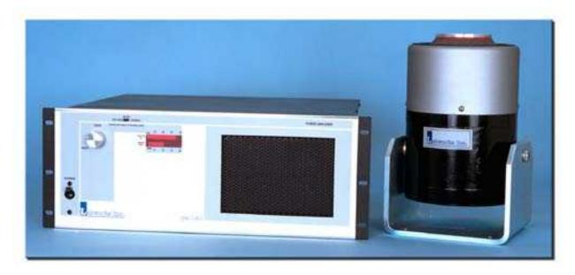
The LW-140-110 is a high performance system capable of very high acceleration (110 g, bare table). It is used for general purpose as well as modal testing. The shaker field supply is integrated into the power amplifier and includes a cooling interlock to protect the shaker..
