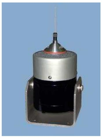
The MT-161 thrusteri s compact size, long stroke and lightweight armature make it well suited for all types of modal testing. The thruster has a compression collet and features a central throughhole suitable for modal stinger and pre-tensioned wire testing applications. The standard shaker trunnion allows the shaker to be operated in any axis from vertical to horizontal. The trunnion base also facilitates bolting the shaker in place for rigid applications or the use of adjustable mounting feet.
