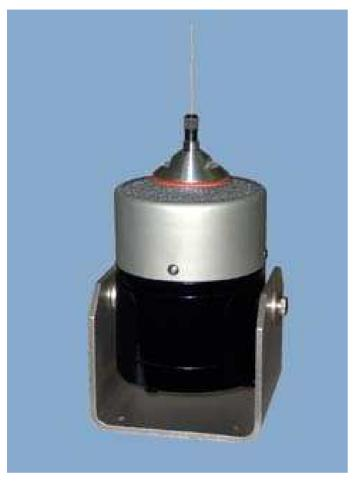
The MT-161 thruster; s compact size, long stroke and lightweight armature make it well suited for all types of modal testing. The thruster has a compression collet and features a central throughhole suitable for modal stinger and pre-tensioned wire testing applications. The standard shaker trunnion allows the shaker to be operated in any axis from vertical to horizontal. The trunnion base also facilitates bolting the shaker in place for rigid applications or the use of adjustable mounting feet.
