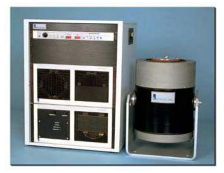
The LW127.123-500 is the largest of the current family of Labworks vibration test systems. Electrodynamic shaker systems consist of a shaker and a matching linear direct coupled power amplifier. Additional components are then added to the basic system to tailor it to your specific needs.
