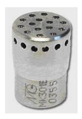
The equalization of the static air pressure between the inside and outside of the cartridge is by means of a capillary tube side-vented. The individual pressure frequency response curves can be convenient measured by using a calibration grid, e.g. UA 0033 by means of the adaptor DB 0264. The cartridge uses the international standard thread 60 UNS which ensures compatibility with a wide range of calibration equipment and measurement devices available from many manufacturers.
